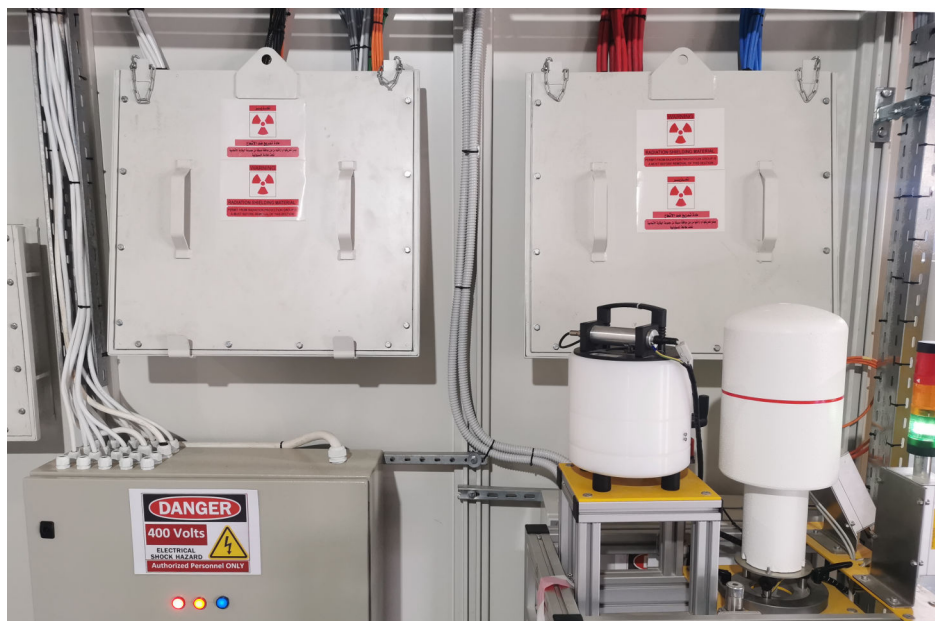
Fig. 18: Radiation shielding chicanes and radiation monitor at BEATS. Modifying, moving or changing in any way the radiation shield as well as any other safety equipment is strictly forbidden.
